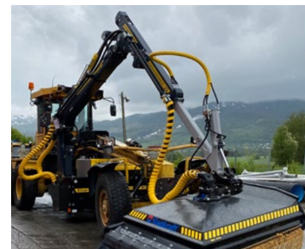
SC8 • A crane with the latest technology, a high crane pillar and protective design. Reach up to 8.5 metres.
