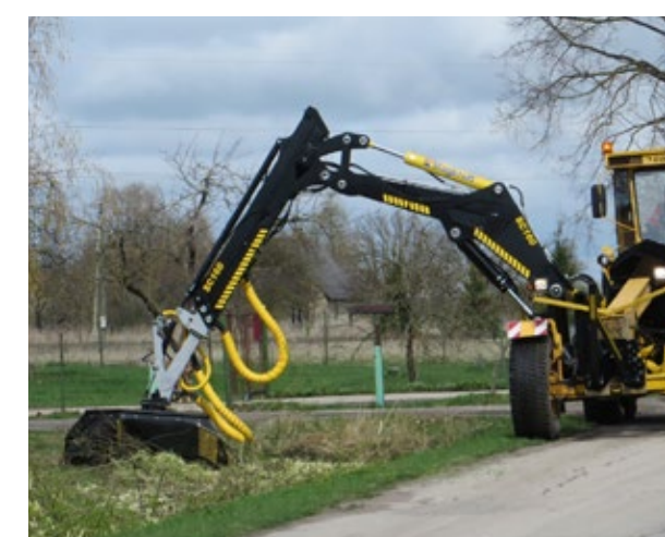
SC160 • A robust crane with a long reach of up to 11 metres with double-telescope technology. For clearing major road networks.
