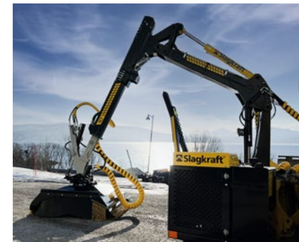
SC7 • A modern crane with a high crane pillar, short main boom and protected hoses. For clearing minor roads.
