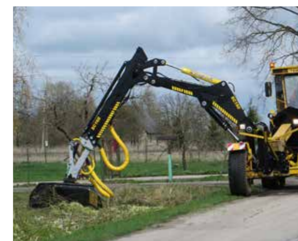
SC160 • A robust crane with a long range up to 11 meters and double telescopic technology. For clearing larger road networks.
