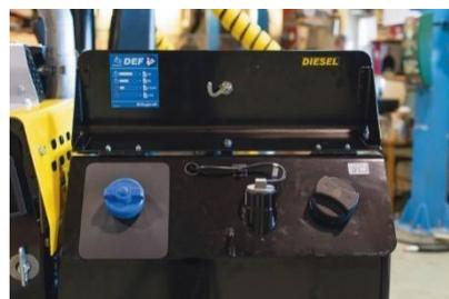
**Tanks.** The fuel tanks of the Power pack have a new panel that is easy to access when refuelling diesel and DEF. Panel is protected by a lockable hood.
