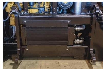
**Oil cooler.** Mounted at the attachment frame with the fans inside which gives optimized cooling and protection.
