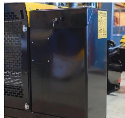
**Fuel tanks.** Tank volumes, 200 litres for diesel and 15 litres for DEF.
