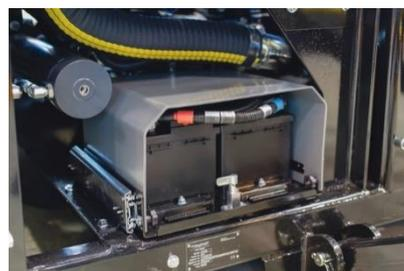
**Batteries.** W180 is equipped with a package of twin batteries. The package is mounted on a sliding shelf for easy access.
