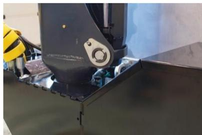
**Crane mounting.** The base of the crane is attached to the machine frame at a low position providing good visibility and centre of gravity.
