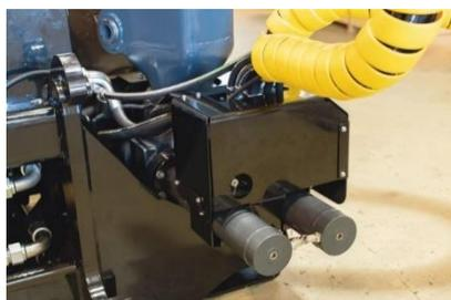
**Main valve.** The valve block is placed close to the base of the crane well protected and easy to access for service.
