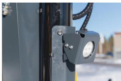
**Lights.** One LED-light is located on the cover for the lift cylinder of the crane.
