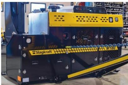
**Engine.** W180 is powered by a new Caterpillar C4.4 diesel engine providing 175 hp. The engine meets the EU Stage V emission regulations.
