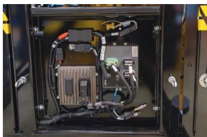
**Electric central.** Located behind a protection hatch at the front of the Power pack. All components easy to access.
