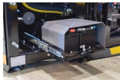
Battery access for service and maintenance well covered by a hood and front hatch.
